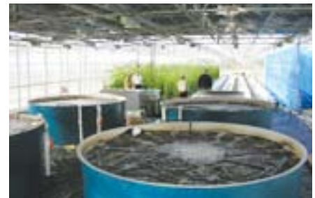
Figure 5. The UVI aquaponic system at the New Jersey EcoComplex at Rutgers University. Effluent from four tilapia-rearing tanks circulates through eight raft hydroponic tanks, producing tomatoes and other crops.
