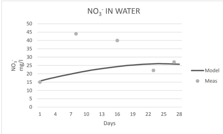
Figure 7. Results for nitrate concentration achieved in water ( $\text{mgN\_NO}_3^- / \text{l}$ ) during 28 days. Dots show the measurements obtained from laboratory and the lines indicated the model predictions using real values of daily feed.
