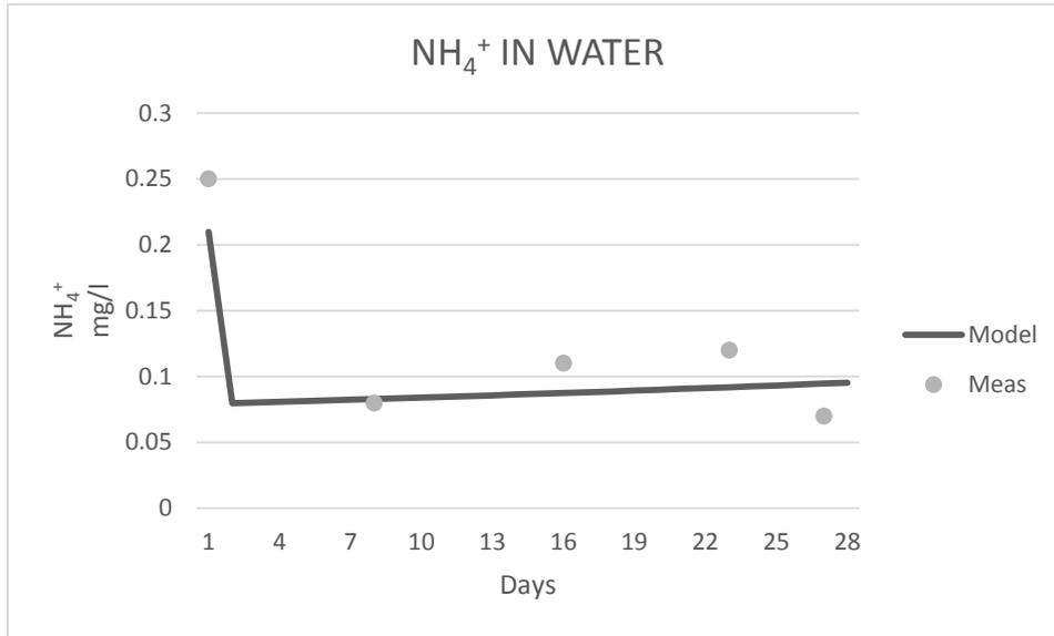
Figure 6. Results for ammonium concentration in water ( $\text{mgN\_NH}_4^+/\text{l}$ ) during 28 days. Ammonium concentrations were simulated using total amount of daily feed (feed) as input. Dots represent the measured concentrations of ammonium and the line indicates the model predicted concentrations for  $\text{NH}_4^+$  in water.
