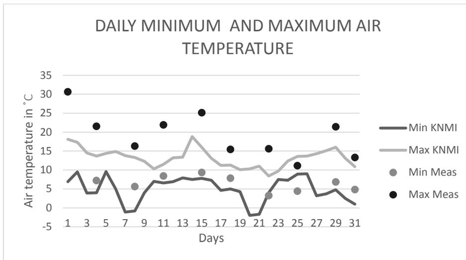
Figure 10. Comparison between minimum and maximum air temperatures. Continuous line refer the downloaded temperature from the weather station in Deelen, Netherlands. Dots refer the air temperature measured twice per week inside the green house.
